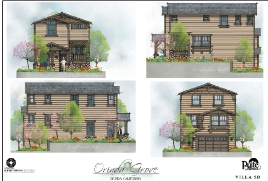
COURTESY OF PULTE HOMES This craftsman style three-story home utilizes the site's natural topography allowing the home to appear to be two-stories from the front and three from the back.
